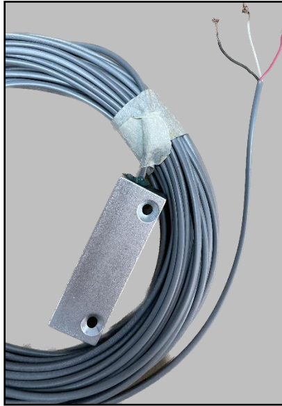
Figure 17. Magnetic Limit switch wires
