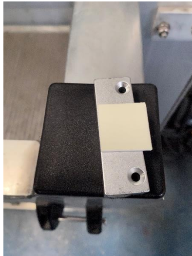
Figure 10. Two-sided tape attached to magnetic component
