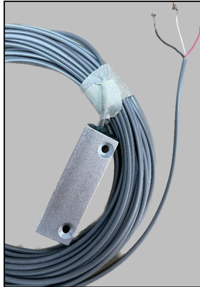
Figure 17. Magnetic Limit Switch wires
