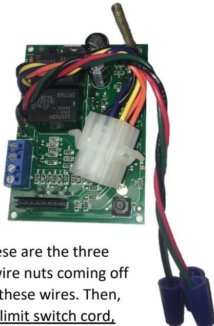
and gel pad. On a 2-stop these are the three wires (five for 3-stop) with wire nuts coming off the control board. Separate these wires. Then, connect these wires to your limit switch cord, color to color. The necessary blue wire nuts will be in the bag with the control box mounting hardware.
